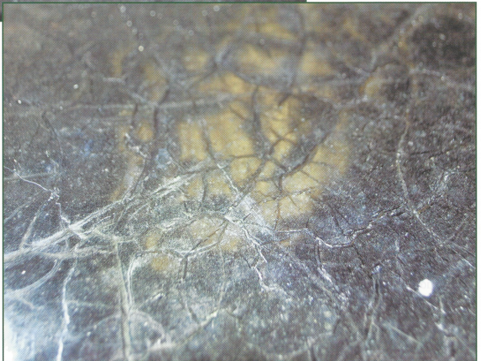
Figure 2 – Surface of SBS-modified bitumen that has been exposed to unfiltered ultraviolet radiation for 1,500 hours.
