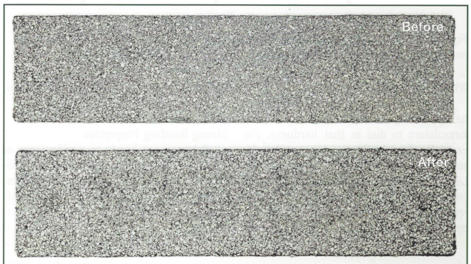
Figure 4 – ASTM D4977 scrub panel of a polyurethane-modified bitumen membrane before and after aging in California for about six months.
