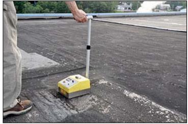
10' grid pattern. Within each grid point, a reading is taken and recorded on a roof plan. The smaller the grid pattern, the more data points are collected. For example, a 10,000 square foot roof with a 10' x 10' grid would require 100 data points. If the grid were 5' x 5', there would be 400 data points.
